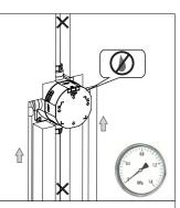
2-2.Plug the top and bottom water outlet with plug, apply a 30min water leakage test under water pressure 10-12 Bar. Make sure there is no leakage.
