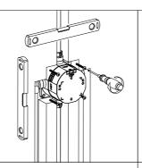
2-1.Get the wall cut accordingly to the instruction, check the horizontality and verticality of the valve box, adjust if necessary. Then fix the valve box onto the wall.
