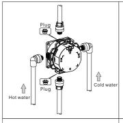
1.Connect the pipe to the water port, Left (H) for hot water and right (C) for cold water, top and bottom for mixed water.Plug the bottom or top mixed water outlet with the block if it's not required to use (single way valve).
