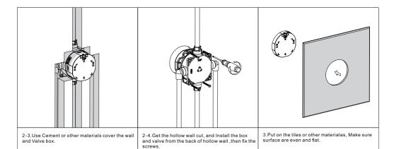
4. Cut the plaster shield and make sure the valve box is at the same lever of the finished wall. 5. Install the fixing plate. (For the valve with 3mm trim plates no need to install this) 6. Open the built-in service stop and flush the pipe.
