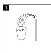
For the first-time install, flush the pipes first by opening the angel valve to run 60s
