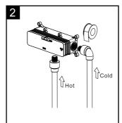
Connect the pipe to the water port, Bottom (H) for hot water and right (C) for cold water
