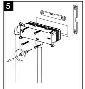
Get the hollow wall cut, and Install the box and valve from the back of hollow wall ,then fix the screws.
