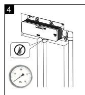
Pressurize the test pipeline for hydraulic pressure to check for leaks Use Cement or other materials to cover the wall and Valve box.
