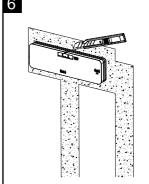
Fill cement to fix the embedded box, cut out the part of the embedded box above the wall.
