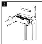
Get the wall cut accordingly to the instruction, check the horizontality and verticality of the valve box, adjust if necessary. Then Fix the valve box onto the wall.
